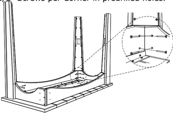
2. Attach (B) Shelf to (C) Legs using 2 - 1 1/2" Screws per Corner in predrilled holes.
