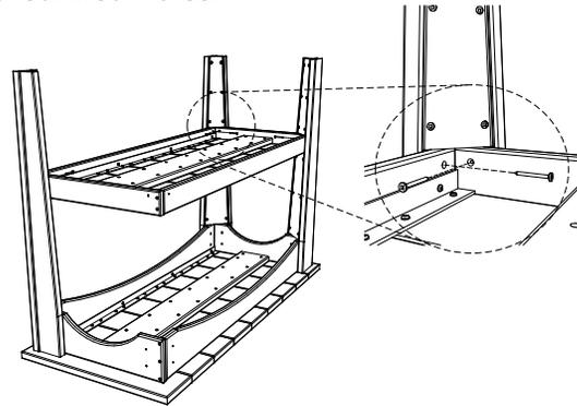
3. Attach remaining (C) Leg to (A) Top & (B) Shelf as shown in step 1 & 2.
