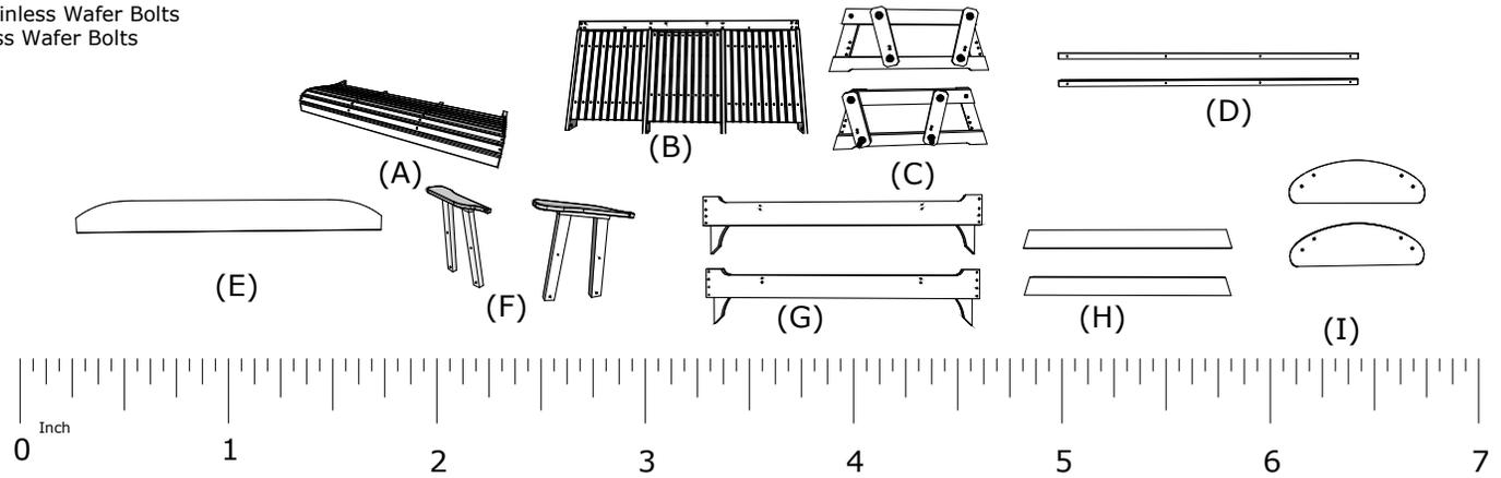
1. Attach (G) Front-Back Crosspieces to (C) Glider Base's Using 14 - 2" Screws per side, be sure to match all numbers & or letters.
