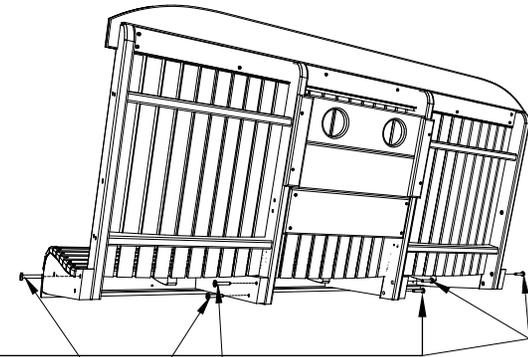
7. Attach Back-Seat Assembly to Armrests using
