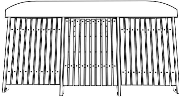
6. Attach Back Assembly to (A) Seat Assembly using 6 - 2" Wafer Bolts, be sure to Match all numbers & or letters, tighten Wafer Bolts with included Hex Key.
