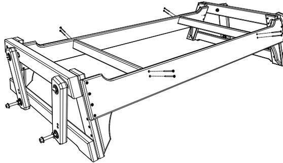
3. Attach (D) Bearing Arm Supports to Glider Base using 4 - 2 1/2" Screws per side, be sure to match all numbers & or letters.
