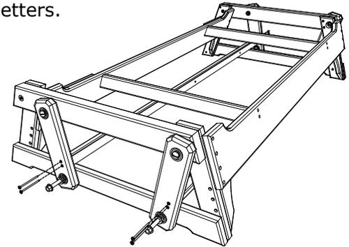
4. Attach (F) Armrests to Glider Base using (2-Washers)&(2-Nuts) per side, be sure to match all numbers & or letters. "Assembly order is Armrest Assembly-Washer-Nut"
