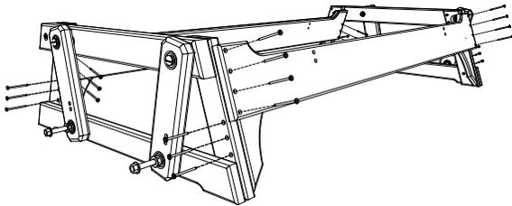
2. Attach (H) Crosspiece Supports to Front-Back Crosspieces using 4 - 2" Screws per side, be sure to match all numbers & or letters.
