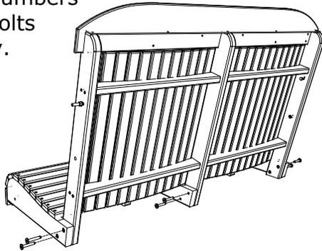
**2. Attach (C) Armrest's** using 1 - 2" Wafer Bolt 1 - 3 1/2" Wafer Bolt 1 - Washer 1 - Nut 2 - 2" Screws & 2 - 1 1/2" Screws per side, be sure to match all numbers & or letters, tighten Wafer Bolt with included Hex Key.
