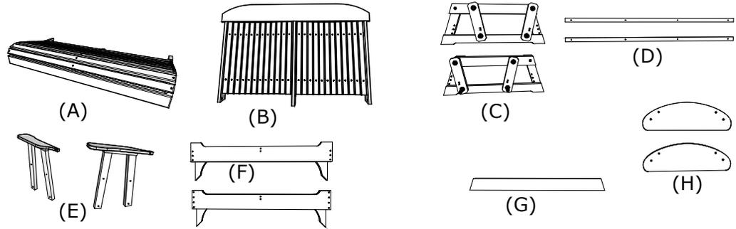
1. Attach (F) Front-Back Crosspieces to (C) Glider Base's Using 14 - 2" Screws per side, be sure to match all numbers & or letters.
