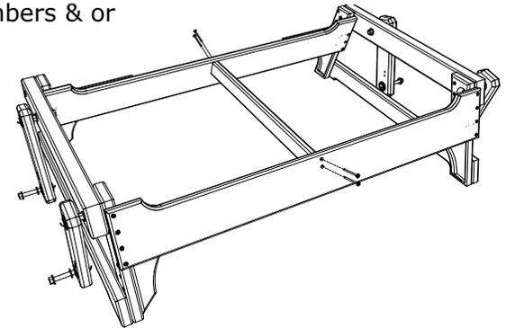
3. Attach (D) Bearing Arm Supports to Glider Base using 4 - 2 1/2" Screws per side, be sure to match all numbers & or letters.
